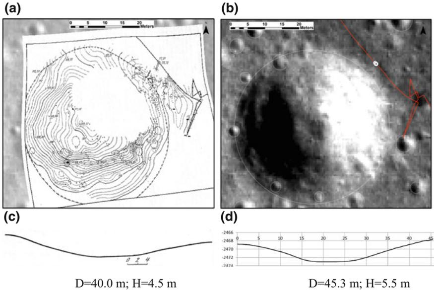
**Fig. 8** Comparison of archive Lunokhod-1 data and recent GIS measurements: (a) topographic map of a small crater (map# 3 from Abramova et al. 1978) referenced to the LROC NAC orthoimage; (b) the same crater identified on LROC NAC orthoimage and a part of rover track identified using the archive map; (c) height profile through the crater from the map # 3; (d) height profile obtained from high-resolution LROC NAC DEM
