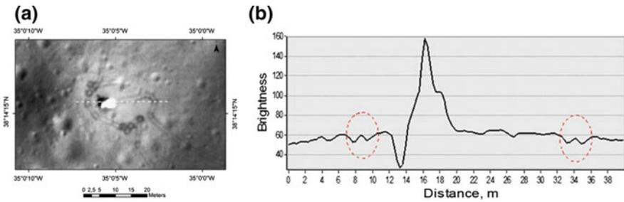
**Fig. 3** Analysis of brightness of Lunokhod-1 wheel tracks: (a) LROC NAC image M175502049 with resolution 0.3 m/pixel; (b) corresponding profile of brightness along transect line with white dashed color on the image. *Note:* W-shaped pattern on the plot representing tracks of left and right rover wheels
