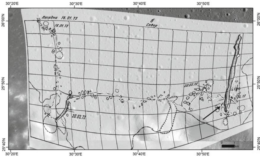
**Fig. 9** Differences between Lunokhod-2 route, digitized in GIS (white), and the route from transformed historic topographic schema (black), produced as the result of analysis and mapping after Luna-21 mission (maximal discrepancy, marked with arrow, is about 80 m)
